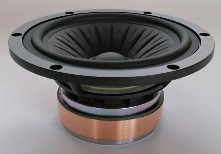
The mid-woofer and woofer are 7-inch modified Eton Orchestra drivers with a characteristically embossed cellulose diaphragm on a rubber suspension. The solid die-cast basket is equipped with our proprietary BAD dampening system. The massive magnet system is vented and grounded. The dust cover has a shape memory - it is resistant to dents. As a result, Bellatrix does not require protective grilles.
